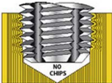
FORMING TAPS Re-arrange the grain of the material.
