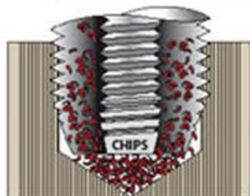
CUTTING TAPS Create chips that interferes with tapping
